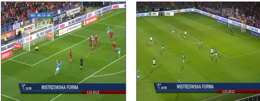
Fig. 3. Two similar consecutive frames of two different shots from different sports events of very similar colour histograms
