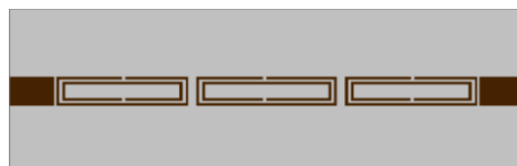
Fig. 16 Layout of three pole microstrip end-coupled split ring resonators filter
