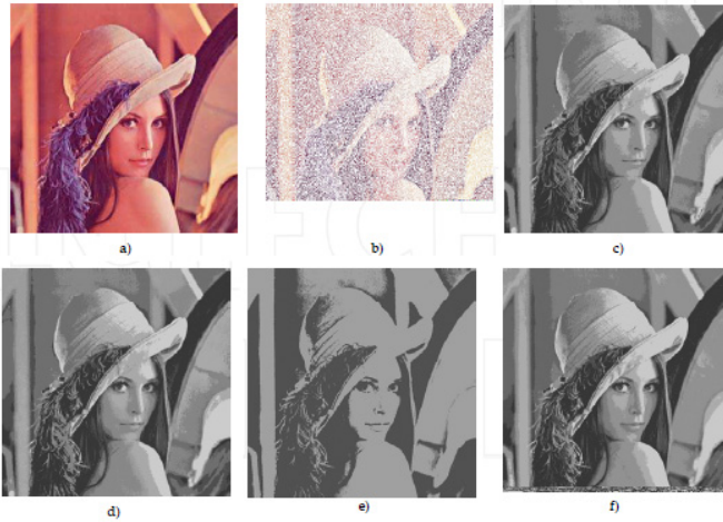
Fig. 7 Image processing using self-learning Fuzzy spiking neural networks. a) Original image; b) Training set (30% of the original image); c) 1st epoch of self-learning fuzzy spiking neural network learning; d) 3rd epoch of self-learning fuzzy spiking neural network learning; e) 3rd epoch of fuzzy cmeans learning; f) 30th epoch of fuzzy c-means learning [16]
