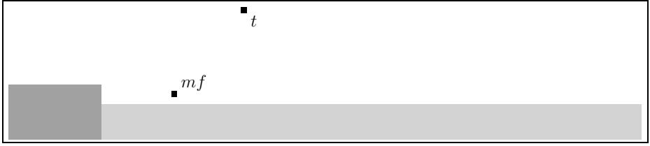
Fig. 5. An example trajectory t and its resulting focus mf using the move focus extension. The functional part is colored in dark gray. Trajectory is assumed to be a toothpaste tube.
