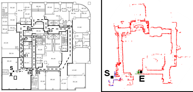
Fig. 5. An accurate map (right) produced using Carmen mapping which uses Monte Carlo Localization based on particle filters and scan matching techniques (Thrun et al. 2001)
