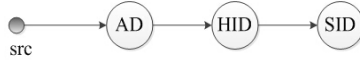
Fig. 2. An example of DAG form address ( src indicates a virtual source of DAG. AD is a 160-bits number identifying an administrative domain. Similarly, HID and SID are 160-bits identifiers presenting a host or a service.).
