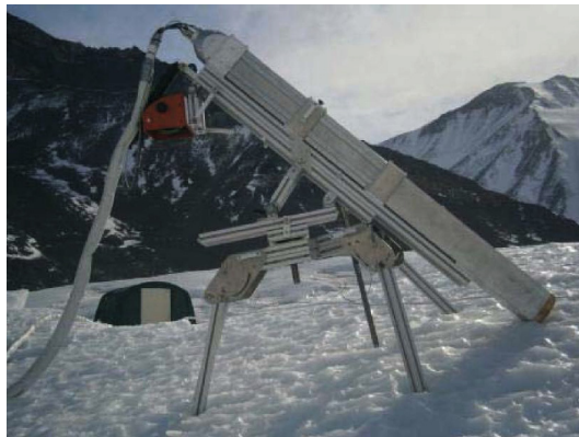
Fig. 1. The maneuverable melting probe “IceMole” in the launchpad on the Commonwealth Glacier in Antarctica. (Figure reprinted from [6].)
