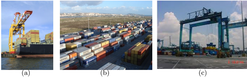
Fig. 1. Container terminal equipment: (a) a Quay Crane (serving a vessel); (b) the container Storage Yard; and (c) a Rubber-Tyred Gantry crane
