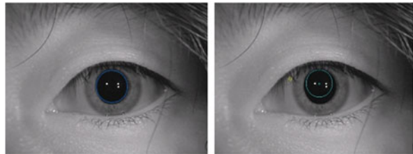
Fig. 58.5 Pupil localization results using the Wildes system (left) and the proposed method (right)
