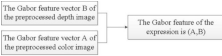
Fig. 76.3 The Gabor feature extraction process
