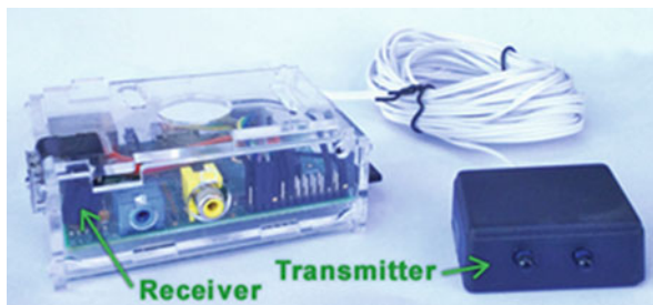
Fig. 119.5 Finished prototype of central point
