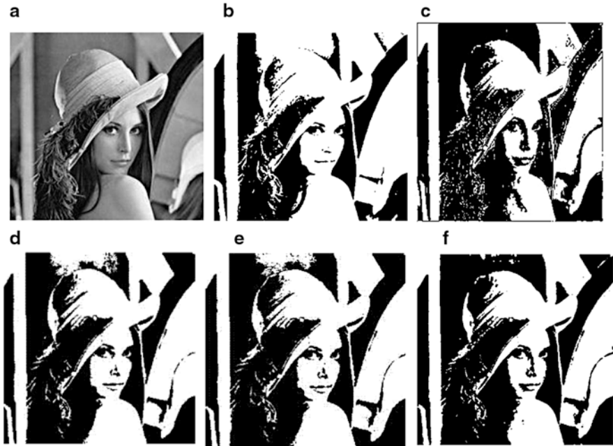
Fig. 81.5 (a) The original image, (b) the method based on OSTU, (c) the method based on normal PCNN, (d) the unit-linking PCNN [3], (e) the GIT-PCNN [1], and (f) RMS-PCNN
