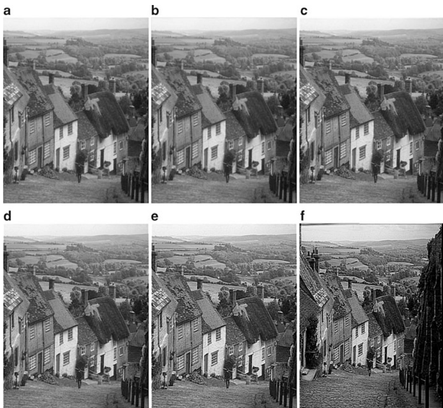
Fig. 66.2 Image enhancement of Goldhill by IFD with different fractional differential orders (a) \nu = 0.0 , (b) \nu = 0.1 , (c) \nu = 0.3 , (d) \nu = 0.5 , (e) \nu = 0.7 , (f) \nu = 0.9
