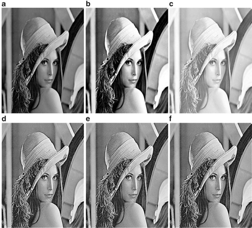
Fig. 66.4 Texture enhancement capability comparison of Lena image (a) original image (b) HE, (c) Retinex mccann99, (d) G-L with \nu=0.8 , (e) R-L with \nu=0.8 , (f) IFD with \nu=0.92
