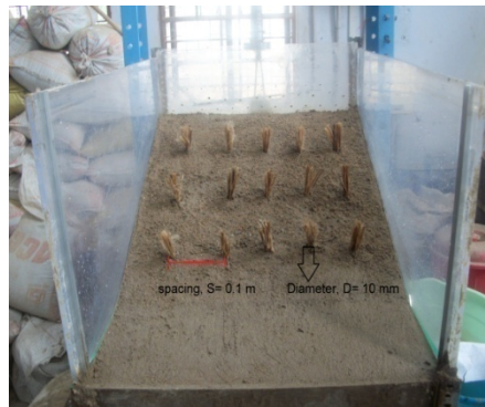
Fig. 4. Front View of a Jute Reinforced Slope
