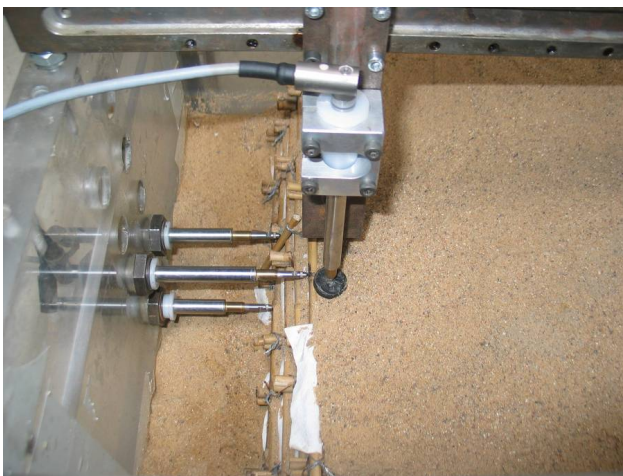
Fig. 5. Measurements arrangements for horizontal and vertical displacement
