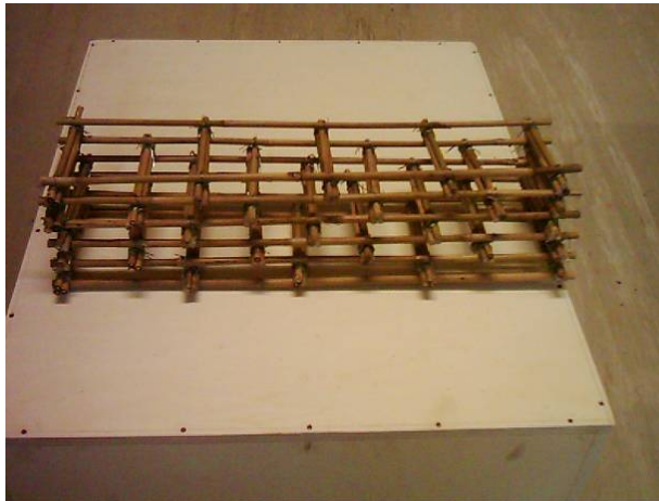
Fig. 3. Model bamboo crib wall
