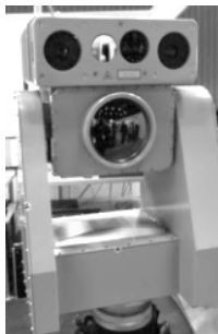
Fig. 1. Sensor head with CCD-C-Z36 TV cameras (Carl Zeiss Optronics GmbH)
