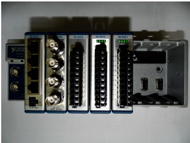
Fig. 6. The NI Compact DAQ chassis, which is being filled with (starting from the left side): Bridge Module (strain gauges), vibration sensors card, analog output card, and two digital signal output and input cards
