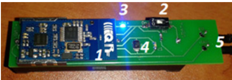
Fig. 4. Picture of the node with mounted transceiver module; 1 – IQRF TR-52D with on-board antenna, 2 – power switch, 3 – power signalization LED, 4 – button for bonding operations, 5 – thermometer wires
