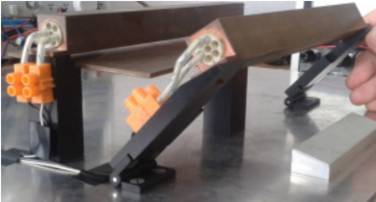
Fig. 4. Photo of the heating elements with the method of the test stand closing/opening
