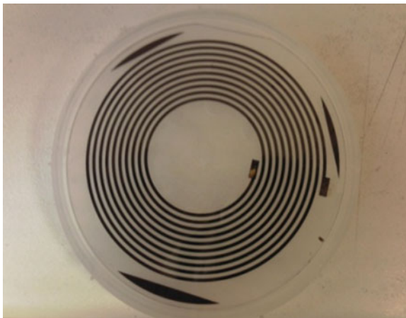
Fig. 7.14 Cryogenic superconducting radiofrequency coil designed to operate at 7.2 MHz and 77 K for use on the low field Niche MRI system. The outer diameter of the spiral coil is 100 mm and there are ten turns of superconducting material deposited on a sapphire base
