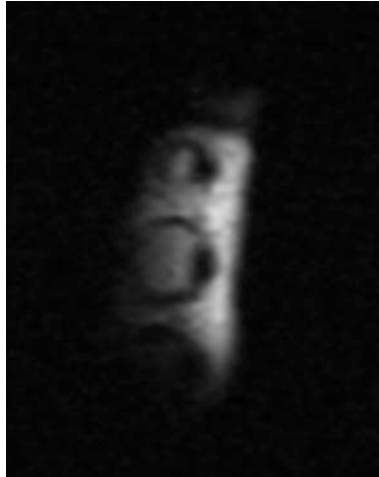
Fig. 7.15 Axial spin echo T1 weighted image acquired through the hand with the cryogenic superconducting coil above cooled to 77 K with liquid Nitrogen in a dedicated vacuum dewar on the 0.2 T Niche MRI system. This type of image could potentially be used with the GRACE method for detection of median nerve stimulation at low field. Note the much improved SNR and geometrical fidelity compared with the EPI image of the wrist acquired at the much higher field strength of 1.5 T shown in Fig. 7.12
