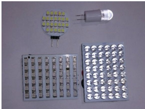
Fig. 9.7 Various types of LEDs available for vision research
