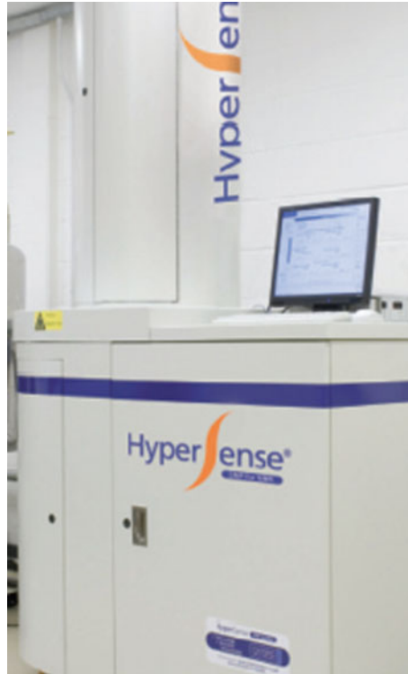
Fig. 7.21 HyperSense dissolution DNP system operates at 1 K and a microwave frequency of 93.5 GHz to polarize a solution of trityl free radical together with a biological substrate which can be metabolized e.g. pyruvate. The DNP system enhances sensitivity for ^{13}\text{C} nuclei by more than 10,000x. It may be possible in future to develop suitable contrast agents to enhance low field dfMRI using this technology. DNP works equally as well for low field strength MRI as the polarization generated does not depend on the field strength of the MR system used for imaging
