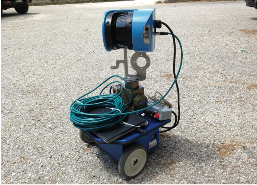
Fig. 8.8 The robotic platform used in the respective work, equipped with a 3D laser scanner and a pan-tilt unit
