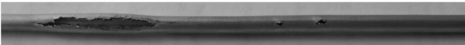
Fig. 6. An example of the formation of defects during the extrusion of the tube
