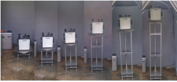
Fig. 4 Gravity measurements at a field station for vertical gradient determination with the use of the stand constructed in the Institute of Geodesy and Cartography, Warsaw
