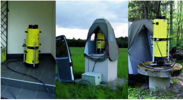
Fig. 4 The A10-020 absolute gravimeter at sites of various types of monumentation
