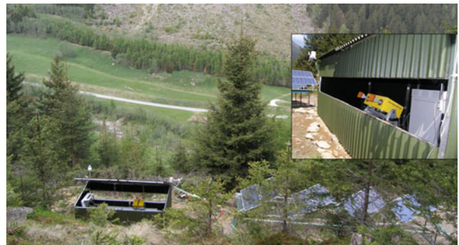
Fig. 3 GB-SAR system IBIS-L facing towards the mass movement ‘Steinlehen’ (S. Rödelsperger)
