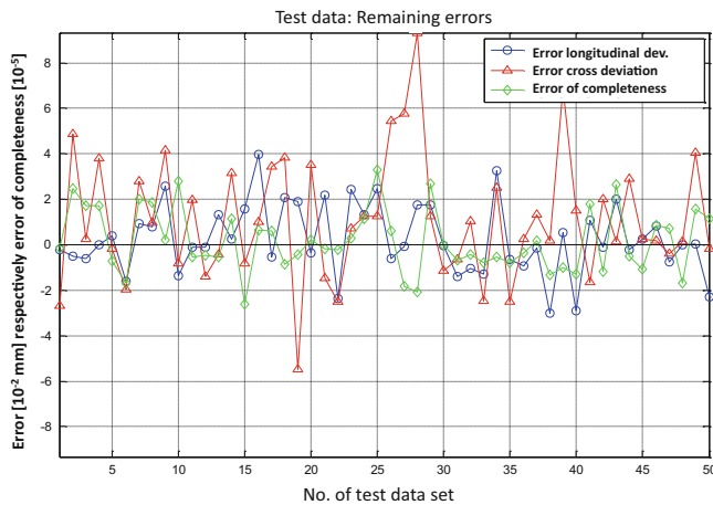
Fig. 3 Polar point determination: Propagation of accuracy and completeness (evaluation data)
