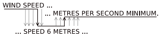
Fig. 1. The concatenation of text chunks in their contexts. The arrow mark all possible concatenation point from which the best (highlighted) can be dynamically selected during synthesis.
