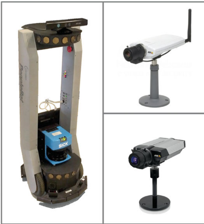
Fig. 15.7 The nodes of the network. On the left , the mobile agent PeopleBot. The robot is equipped with a laser range-finder SICK LMS200 and a Kinect. On the right , two different AXIS cameras: on the top , a Mpixel Axis IP color camera with 1,280 \times 1,024 . On the bottom , an Axis IP color cameras with a 640 \times 480 pixel camera
