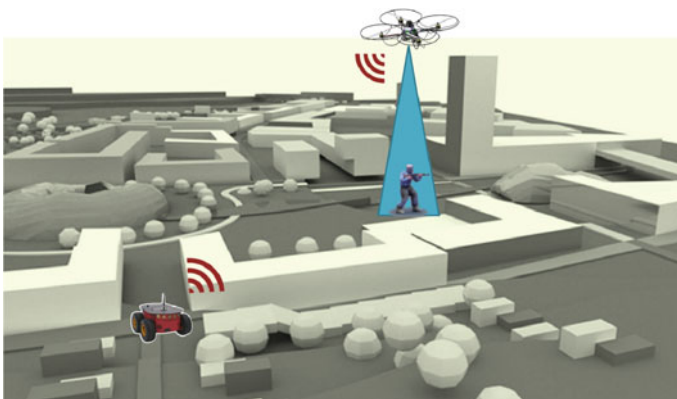
Fig. 14.2 The concept of cooperative target tracking using an unmanned aerial vehicle and an unmanned ground vehicle
