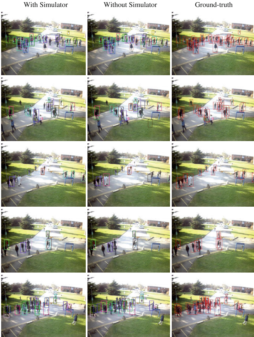
Fig. 13.4 Some sample images for view 2. The left column are the results from the tracker with simulation. The middle column are the results without simulation. The right column are the corresponding ground-truth by annotation. Pedestrians who only appear in one view are not shown
