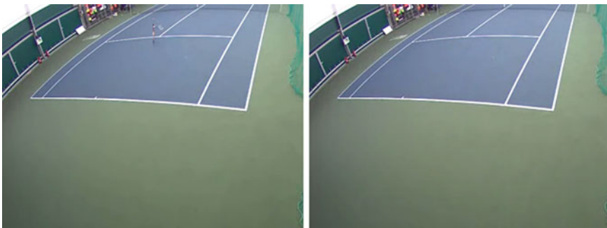
Fig. 9.8 Example of incorrect ( left ) and correct ( right ) background using the junction of portion from different frames background generation method
