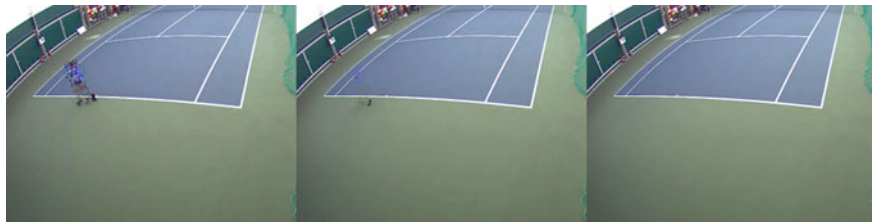
Fig. 9.4 Background generation process for the median-based background generator. From left to right , background obtained using 10, 30, and 90 frames for the median, respectively
