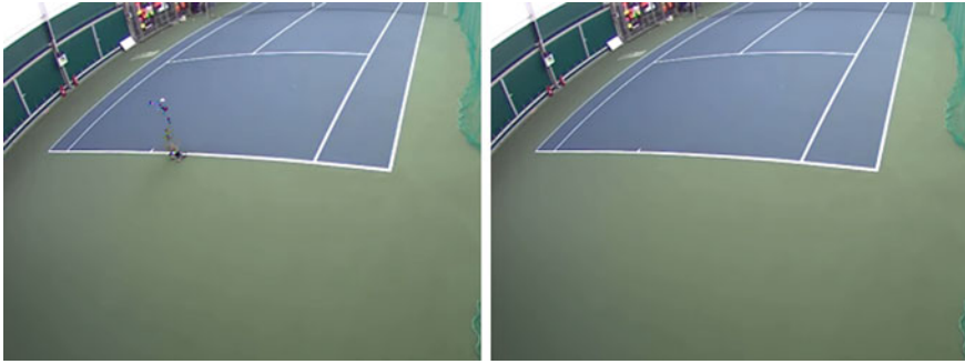
Fig. 9.6 Example of incorrect ( left ) and correct ( right ) background using the mode-based background generation method
