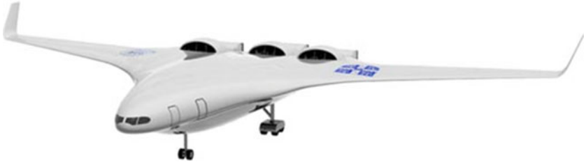
Fig. 1.4 The SAX-40 BWB configuration (© Silent aircraft consortium)
