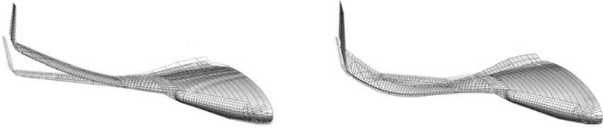
Fig. 3.56 First two symmetric elastic mode shapes
