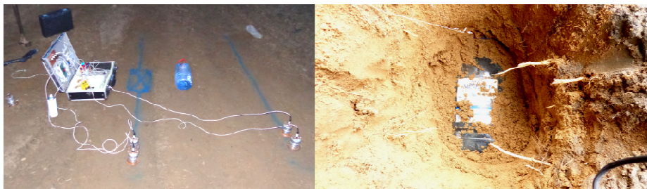
Fig. 3. Heterogeneity is imitated by the plastic water bottle. Measurements were performed along the profiles denoted by blue lines (shown on the left). The water bottle has placed at the depth of a half of the meter (shown on the right).
