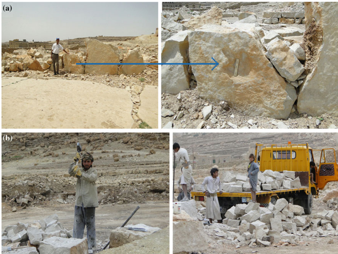
Fig. 18 a Rock layers containing the prints for the purposes of construction (ruler = 20 cm). b Limestone rocks are a major source of building stone in the region
