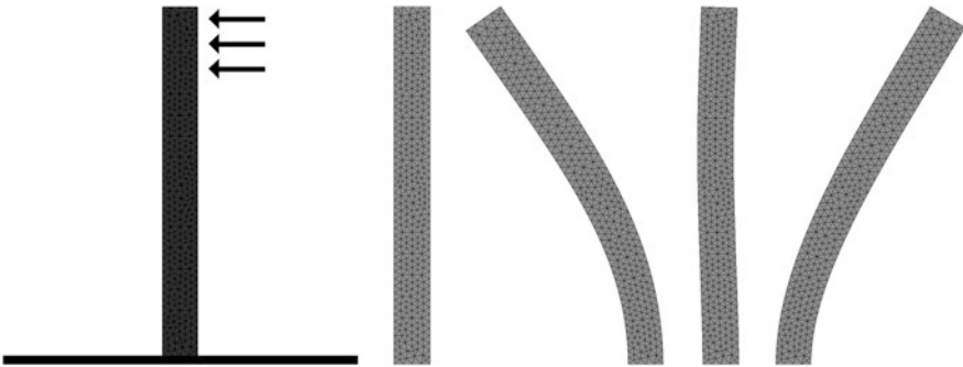
Fig. 1 Schema of the model problem ( left ) and the visualization of the evolution of the displacement function \mathbf{u} at the time instants t = 0, 0.01, 0.02, 0.03 \text{ s}
