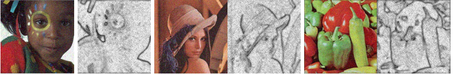
Fig. 1. The color homogeneity maps (right in each pair) for original images corrupted with mixture of Gaussian ( \sigma = 10 ) and impulse ( p=0.1 ) (left in each pair)
