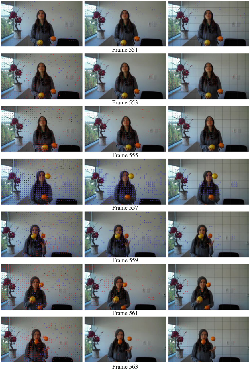
Fig. 9.5 The LMVs estimation in static scene from video sequence “EllenPage_Juggling.avi”: all calculated LMVs are in the left column; the reliable LMVs based on the TSK model are in the middle column; the reliable LMVs in the selected cells of imposed grid are in the right column
