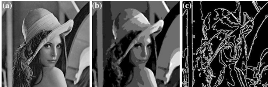
Fig. 2.4 The simplification of image by the connected filter: a the source grayscale image, b the image filtered by connected version, c corresponding frame partition
