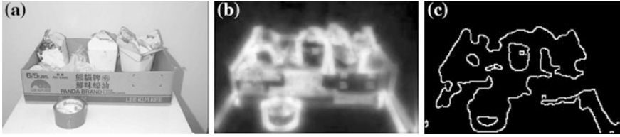
Fig. 8.3 Example of boundary extraction. a An original image courtesy of Caltech [28]. b A saliency map generated by CASD. c Edges from saliency map
