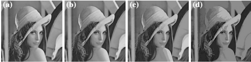
Fig. 2.24 Projective monotonous DP-opening of grayscale image by level set tree with regularization parameter \alpha producing different number of support regions n : a \alpha = 0 , n = 1,584 , b \alpha = 1,000 , n = 120 , c \alpha = 10,000 , n = 24 , d \alpha = 100,000 , n = 8
