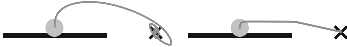
Fig. 2 On the left , the pedestrians motion is governed by the Social Force Model. The pedestrian circles around the target ( cross ). This is because of inertia: the pedestrians velocity vector does not point directly to the target. In contrast, the Gradient Navigation Model directly changes the pedestrians velocity direction ( right figure )
