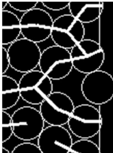
Fig. 2 Example of contact force network. The particles move from left to right side of the picture. When two particles have penetrated, the white line that connects two particles is depicted, and the system shows the network structure. In this calculation, the thickness of the line does not depend on the magnitude of force for simplicity. Note that the shape of the particles ( circles in the picture) is depicted in this example picture for clarification, but it is not drawn in the actual calculation
