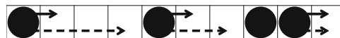
Fig. 1 Schematic view of TASEP and SFI model ( V_{max} = 3 ) with parallel-update rule and periodic-boundary condition. Particles move to their target cells with the probability p in one time step. Solid and dashed arrows represent movements of the particles in TASEP and SFI model ( V_{max} = 3 ), respectively
