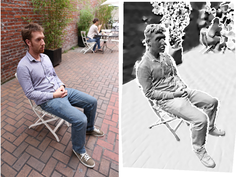
Fig. 1. Example of the proposed surface reconstruction in action: one of three handheld images (left) and surface output (right) rendered with Oren-Nayar shading [27]
