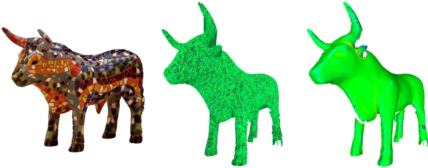
Fig. 9. Left to right: one of five 2746 \times 1832 images of a ceramic bull figurine taken with a telephoto lens, reconstruction from stereo correspondences using elas [12], reconstruction at \alpha = 4 and scale 4 using this work. Rendered with mean curvature colorization, best viewed in color.
