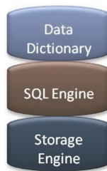
Fig. 3. Components of a DB Engine like postgresSQL: starting point for MPP SQL
