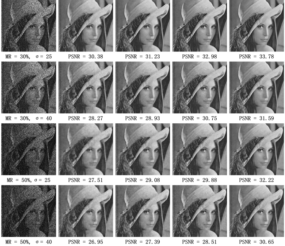
Fig. 3. From left to right: corrupted images, restored results of TV-based method, NL-Means, BM3D and our approach. Our approach outperforms the others for all the situations especially for the examples with high missing rates.
