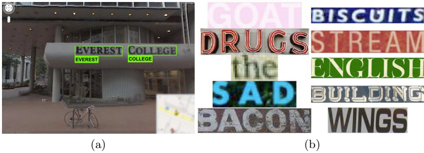
Fig. 1. (a) An end-to-end text spotting result from the presented system on the SVT dataset. (b) Randomly sampled cropped word data automatically mined from Flickr with a weak baseline system, generating extra training data.
