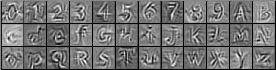
Fig. 3. Visualizations of each character class learnt from the 37-way case-insensitive character classifier CNN. Each image is synthetically generated by maximizing the posterior probability of a particular class. This is implemented by back-propagating the error from a cost layer that aims to maximize the score of that class [43, 17].
