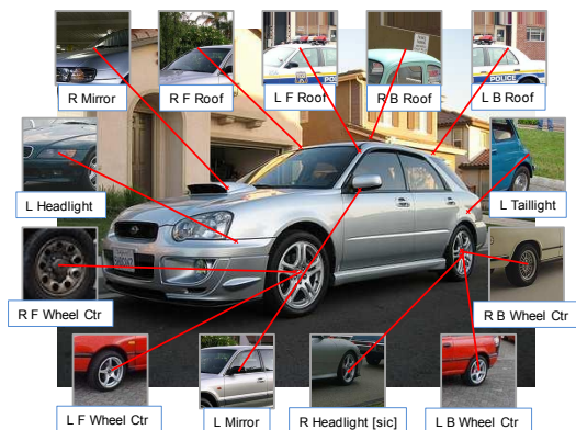
Fig. 9. An example of keypoint transfer. For each predicted keypoint, we show a patch from the image where that keypoint was transferred from. These correspondences are discovered without any supervision. Note that multiple different labels are predicted for the wheel centers. This happens because our algorithm finds all wheels somewhat visually similar, and proposes as many correspondences as possible.
