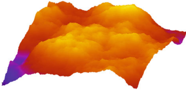
Fig. 12.9 Topography picture of a surface produced by the eroding process described in Fig. 12.8 after removing 76,290 layers of blocks. The surface plane consists of 2,048 \times 2,048 blocks. The surface is self-affine fractal with the Hurst exponent H = 1 (or fractal dimension D_f = 2 ) (see Fig. 12.10). The width of the removed particles (or blocks) is a = 0.1 \mu\text{m} . The surface has the rms roughness h_{\text{rms}} = 2.1 \mu\text{m} and the rms slope \kappa = 1.04
