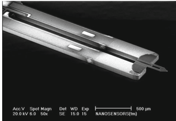
Fig. 18.3 SEM image of Akiyama probe. Copyright by NanoWorld AG
