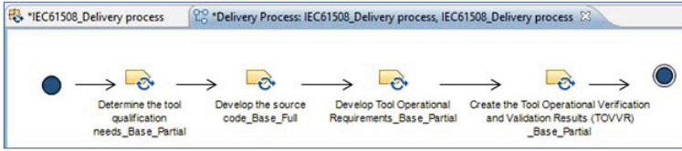
Fig. 7. Derived IEC 61508-compliant tool qualification process
