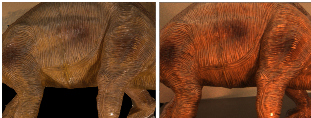
Fig. 4. Dinosaur model: Pre-acquired surface map (left), rendered from the correct viewpoint, matching the actual camera image (right). White dot fiducial on back leg.
