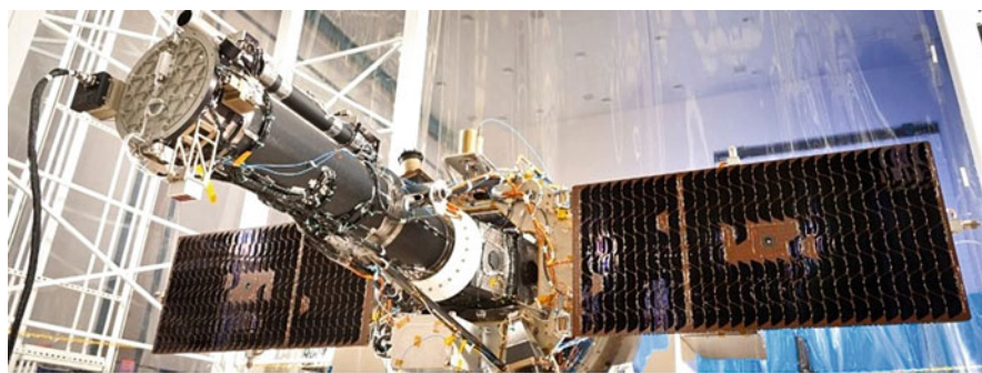
Fig. 1.18 A view of the IRIS instrument (telescope and spectrograph) mounted on the S/C. Note the guide telescope on top of the telescope (courtesy A. Title)
