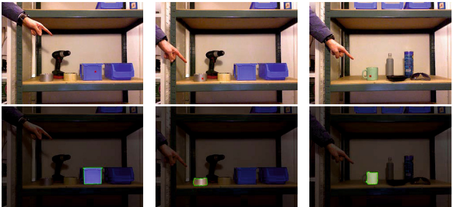
Fig. 7. Pointing and segmentation results of various domestic and industrial objects
