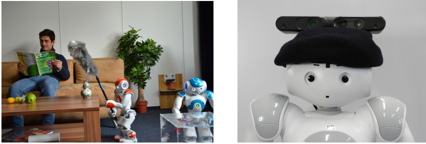
Fig. 1. (Left) Final scenario to be used and (Right) NAO robot with RGB-D device
