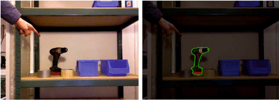
Fig. 2. Extraction of indicated object by pointing gesture
