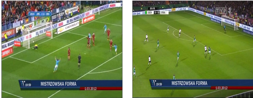
Fig. 4.6 Two clearly different consecutive frames of two different shots from different sports events but, however, of very similar color histograms
