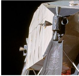
Fig. 1. RCT blocks on the Apollo Lunar Module (Source: http://www.hq.nasa.gov/office/pao/History/alsj/a14/AS14-66-9254HR )
