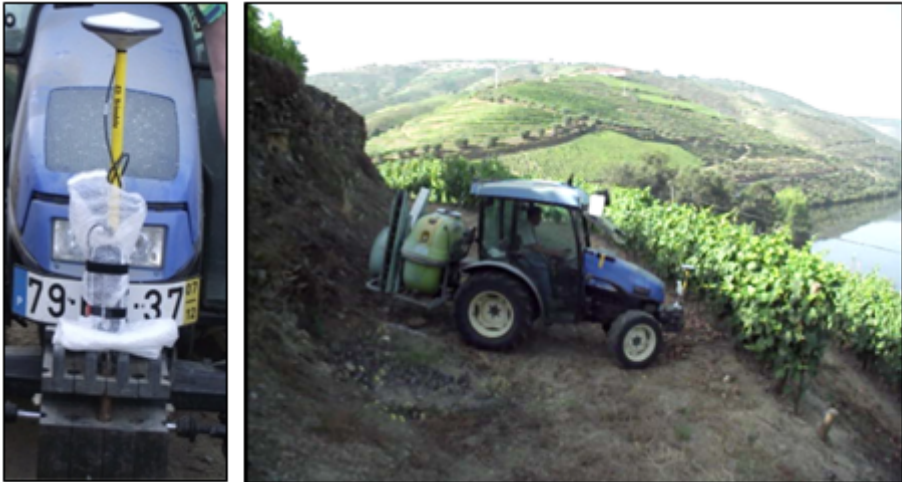
Fig. 3. GNSS Equipment assembly (left) and tractor maneuvers (right)
