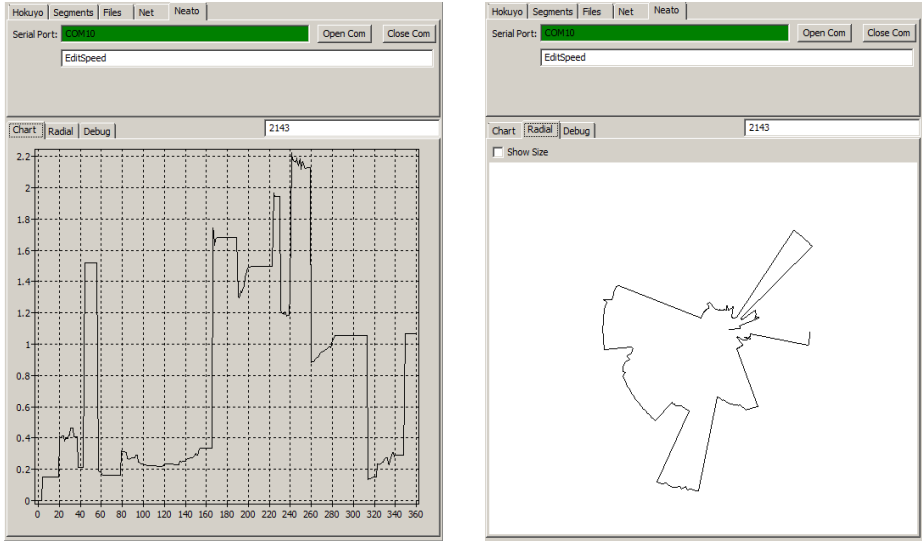
Fig. 3. Developed application that interfaces and acquires data from Piccolo Lidar
