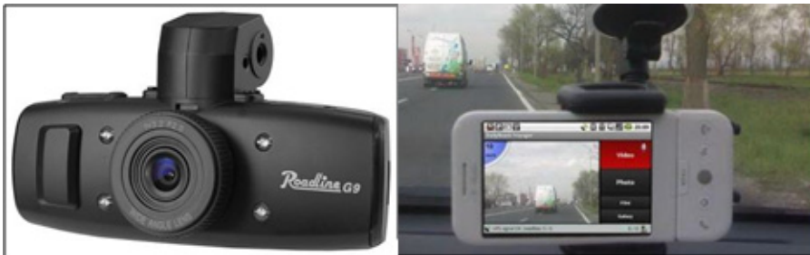
Fig. 1. VMSC (left) and smartphone acting as a VMSC (right)
