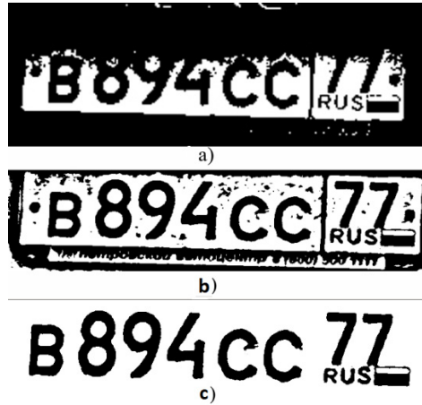
Fig. 10. License plate post processing: a) with global threshold b) with local threshold, c) after contour filtering
