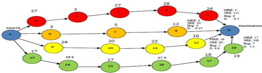
Fig. 4. BBU-AODV route setup from node S to node D
