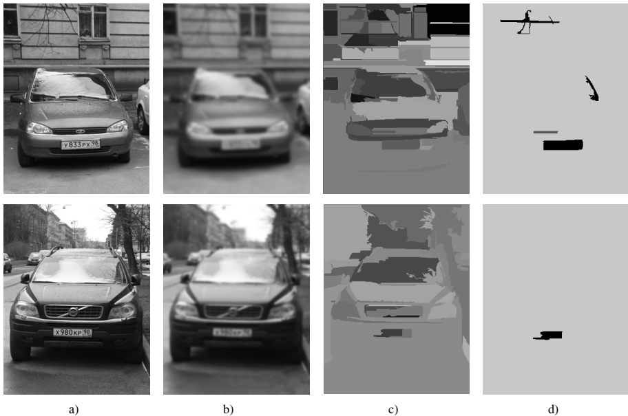
Fig. 1. Image processing stages: a) input images; b) after Gaussian smoothing; c) quantized images; d) segmentation of plate-candidate
