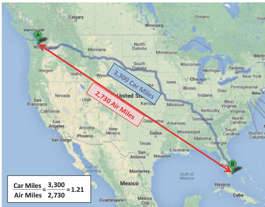
Fig. 1.12 Car (blue-grey) vs. air (red) routes from Seattle, Washington to Miami, Florida. (Adapted from Google Maps)
