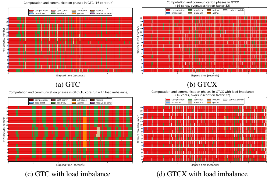
Fig. 4. Computational phase diagrams for GTC and GTCX with and without a synthetic load imbalance on 16 cores are presented here. For GTC, a load imbalance results in the idling of resources until the slowest process catches up with the rest of the processes in its computation as seen by comparing (a) and (c). There is also an increase in idled resources for GTCX in the presence of a load imbalance; however, the difference between (b) and (d) for GTCX is not as substantial as that for GTC due to the ability to overlap computational phases and implicitly load balance.
