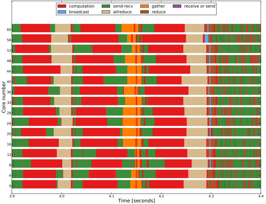
Fig. 2. The phases of computation for a portion of a second in a GTC (MPI based) simulation on 64 cores. The phases for every fourth processor are plotted in the vertical axis for GTC. There is no oversubscription in this case; blocking MPI collectives ensure the computational phases do not overlap significantly. For comparison with GTCX (HPX-3 based), see Figure 3 where the computational phases for the operations corresponding to those here are plotted.
