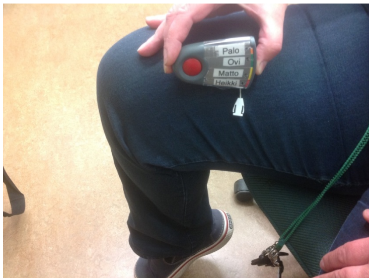
Fig. 5. The vibration alerting system carried by hearing impaired employers on the body. There are four different alerts, all with their own purpose. In this case they are: door, approaching person within office, a special alert for one of the colleagues and fire alarm. Fire alarm also alerts about general alerts in the building. The vibration is similar in all four scenarios, but the light display shows which one of the alerts it is.
