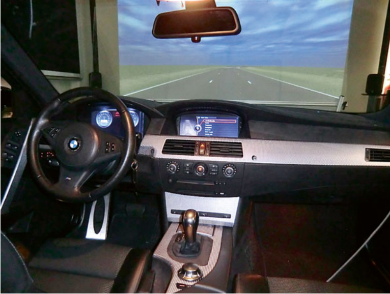
Fig. 32.3 The driving simulator used for the evaluation of the in-vehicle mode ( online mode ) of the framework. It is the real cockpit of a BMW 5-series. The framework controls parts of the dashboard and the display on top of the center stack, and can log most controls by monitoring the vehicle's CAN bus
