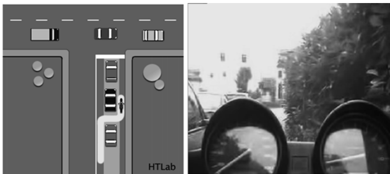
Fig. 6.3 The interstitial room available to a motorbike seen from above ( left ) and from the riders' camera ( right )
