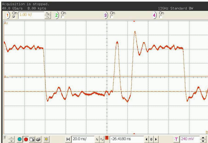
Fig. 6. Inserting a glitch into a 7.37 MHz clock coming from a target device.
