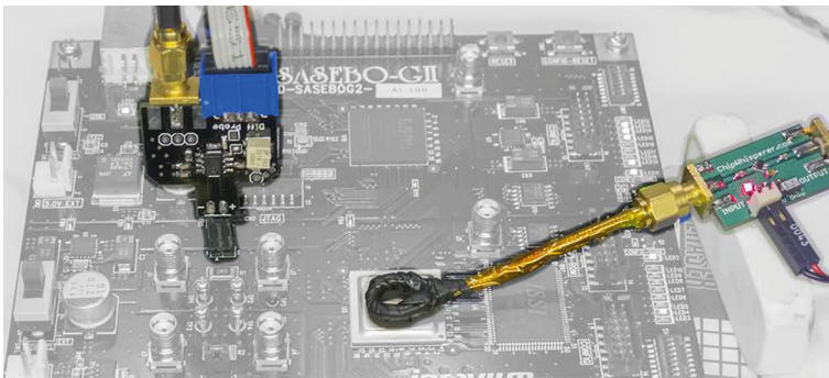
Fig. 4. Beyond capture hardware, design for a differential probe and H-Field probe with LNA are available.
