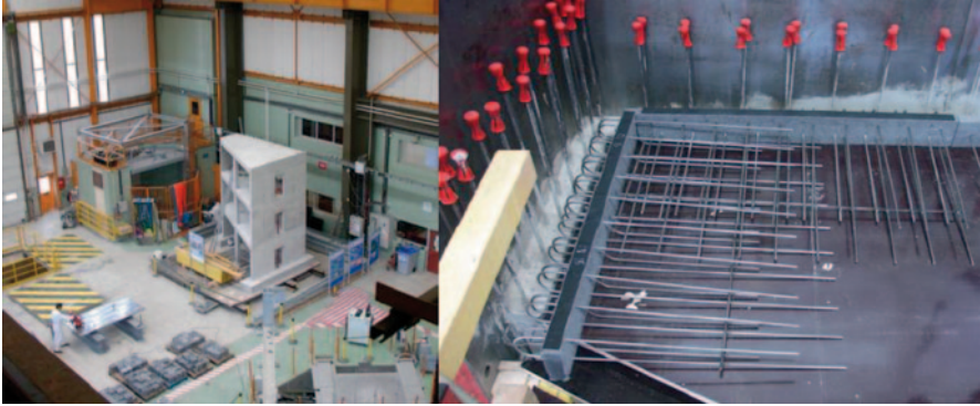
Fig. 19.4 View of ENISTAT specimen and installation of thermal break elements at the SEMT/EMSI laboratory in CEA
