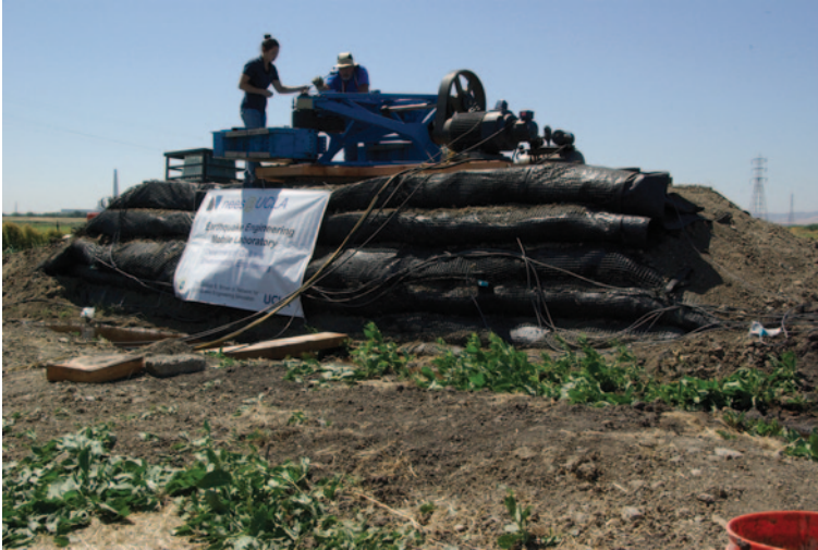
Fig. 1.3 NEESR-II: evaluation of seismic levee deformation potential by destructive cyclic field testing NSF award #: 0830081, PI name: Scott J. Brandenberg, Co-PI: Jonathan P. Stewart, Robb E.S. Moss, Research Sites: University of California, Los Angeles and University of California. (Reproduced by permission of PI: Prof. Scott J. Brandenberg, Department of Civil and Environmental Engineering, University of California, Los Angeles)
