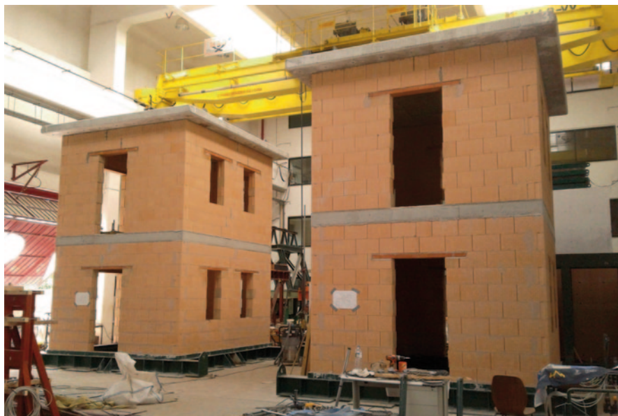
Fig. 15.1 Mock-up A and B in the test lab before testing
