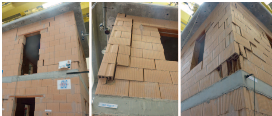
Fig. 15.8 Observed collapse mechanisms of symmetric Mock-up A
