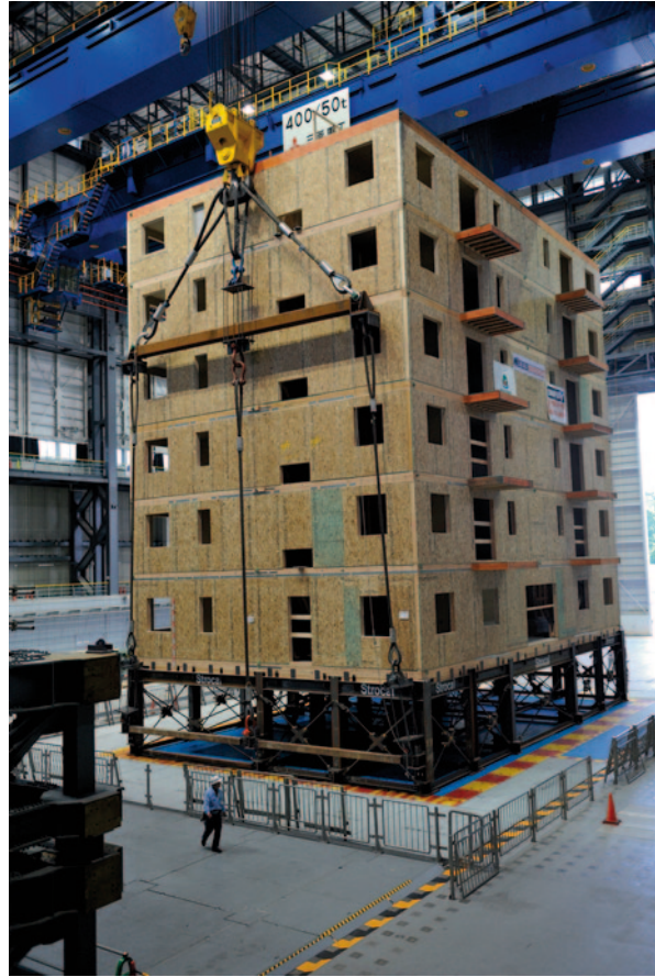
Fig. 1.7 Testing the NEES-Wood Capstone building on the E-defense shake table. (Reproduced by permission of PI: John W. van de Lindt, Colorado State University)
