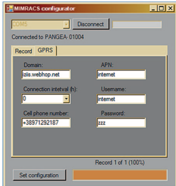
Fig. 36.3 MIMRACS configurator panel for setting GSM and GPRS settings
