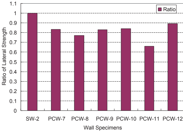
Fig. 23.5 Ratio of lateral strength of wall specimens
