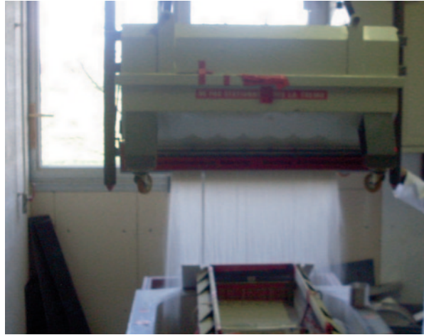
Fig. 29.6 Sand pluviation system
