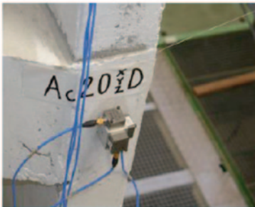
Accelerometers in X-Y-Z directions
