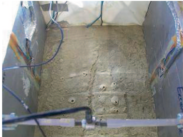
Fig. 33.12 Test PWU2. Photograph of the model, showing sand boils between the two walls, at dredge level
