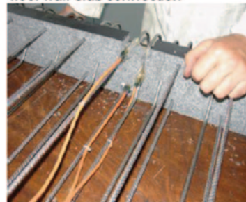
Strain gages on thermal break elements
