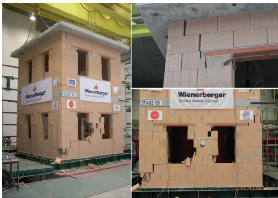
Fig. 15.9 Observed collapse mechanisms of asymmetric Mock-up B
