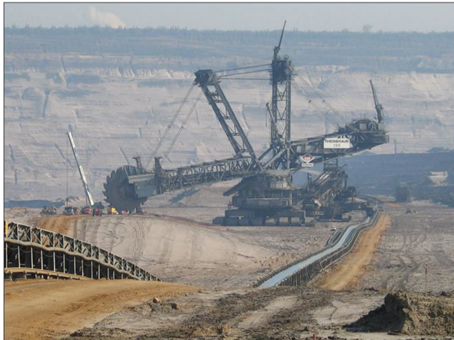
Fig. 1 Rotary excavator RB 289, by manufacturer Orenstein and Koppel (O&K)
