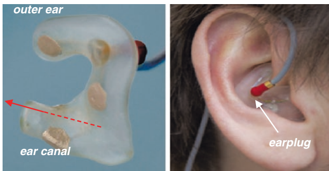
Fig. 2 Left The right Ear-EEG earplug with electrodes visible and an arrow indicating the direction in which it enters the ear canal. Right The earplug inserted in the right ear
