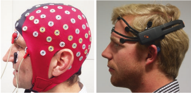
Fig. 1 Left A 128-channel ‘stationary’ EEG system (asalab, by ANT neuro) and right a wearable system (Emotiv EPOC headset)
